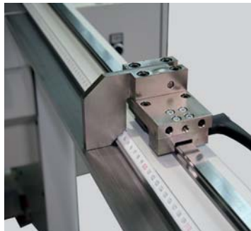
Extended angle gauge on the right with scale incl. lateral flip gauge on linear guide
