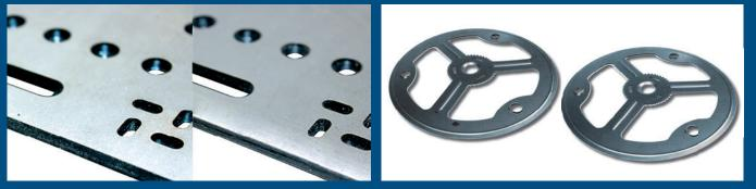
Typical punched and laser-cut parts for the EdgeRacer<sup>®</sup>.
